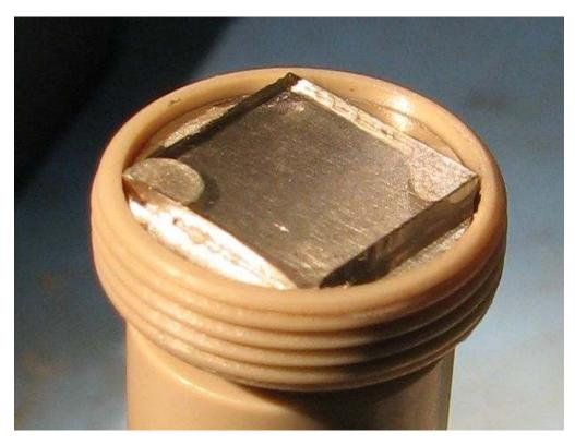
**Figure 24.6.:** Typical square sample of ITO on glass substrate. Note the dabs of silver paint at the corners which electrically connect the sample top surface to a metal disc carrier.
