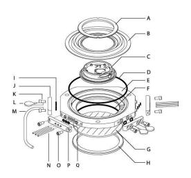
Figure 14.2.: Complete Parts breakdown of the Closed Fluid Cell.
