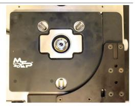
**Note** Base plates prior to 2009 usually only have divots for the rear legs. Current model base plates have one groove for each leg.
