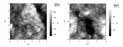
Figure 18.6.: Sample images taken in AC mode at temperatures approaching 400C.
