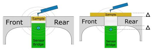
(a) Side view of a small sample between the pole faces.
