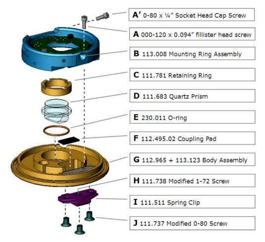
Figure 11.2.: Standard cantilever holder, exploded.
