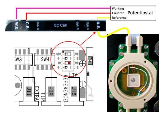
**Figure 24.14.:** The fluid filled reference electrode Connected to the Junction Box and dip switch 5,3 set to ON to connect to the potentiostat reference electrode.
