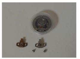
The standard spring clip that holds the cantilever is slightly magnetic and leads to unwanted field gradients and poor magnetic field sensor readings. We have provided a nonmagnetic clip made of beryllium copper that can be substituted when using the VFM.
