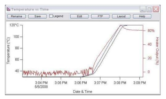
**Figure 20.5.:** The latter part of this graphs shows the heater power as the temperature ramps up to 120C.
