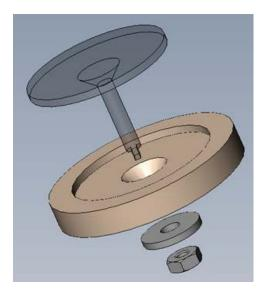
Figure 24.23.: Experimental Parafilm sample mount 939.018.
