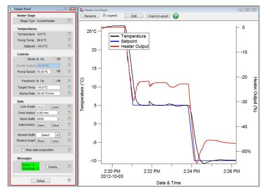
**Figure 20.4.:** Test of the Bioheater. What you might expect to see. Note that the temperature control will be less noisy if the cell is covered. You'll discover this when using it inside the AFM.
