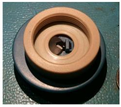
(a) Cantilever holder clearance when using the thin film sample mount. Note that for optimal clearance the cantilever does not land in the center of the visible part of the sample.
