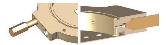
**Figure 24.9.:** A view of a fluid port fitting on the left. The cutaway view on the right shows the straight through port in the back (for fluid or wire feedthrough) and a cutaway of the fluid only port, designed to drain the fluid from the bottom of the cell.
