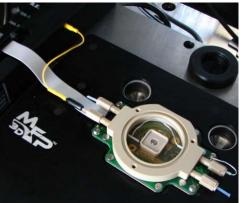
Asylum Research supplies an Ag-AgCl fluid filled (3.4 M KCl) reference electrode which can be inserted through one of the two fluid ports. The Electrode has a PEEK barrel, a proprietary inert frit, and requires no maintenance. In other words, it cannot be opened and it never needs to be filled. It can be stored dry and may only required soaking in de-ionized water before use.
