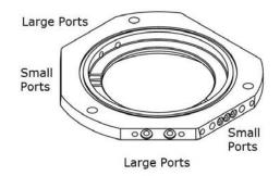
**Figure 14.5.:** 4 Large Fluid ports accept 1/16" OD tubing and 6 small ports accept 20 gauge hypodermic tubing or needles (0.036" OD).
