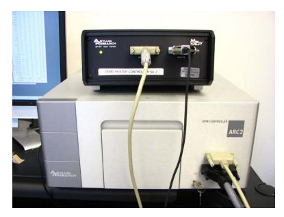
**Figure 16.2.:** Environmental Controller connected to an ARC2 AFM Controller with a DB25 cable with interrupted shield (see gray sleeve close to one end). A temperature stage is plugged into the Environmental Controller.
