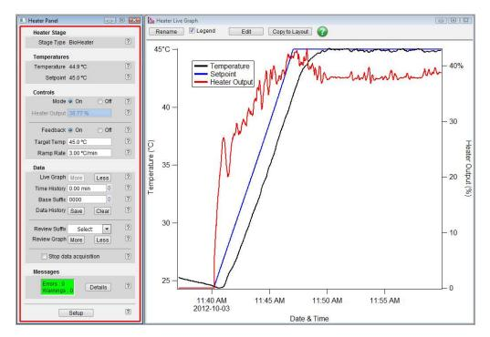
**Figure 17.3.:** Test of the Bioheater. What you might expect to see. Note that the temperature control will be less noisy if the cell is covered. You'll discover this when using it inside the AFM.
