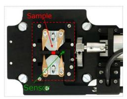
(a) Sample and sensor positions for the original VFM.
