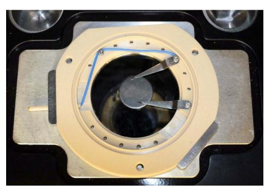
Figure 15.1.: The electrical closed cell in a typical configuration.
