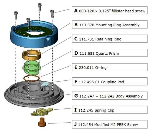
Figure 11.4.: PEEK Cantilever Holder Exploded.
