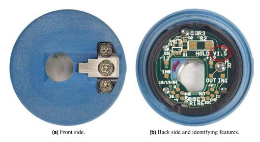
Figure 11.1.: Standard Cantilever holder.
