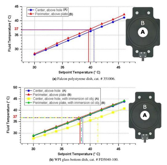
Figure 23.3.: Fluid temperature as a function of controller setpoint, i.e. Target Temp.
