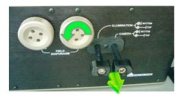
**Note** Once you have an image of the cantilever you can adjust the diaphragms for better contrast.
