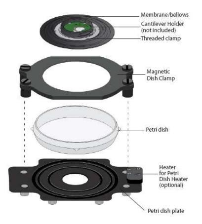
Figure 22.2.: Schematic diagram of complete assembly, in this particular case with the Petri Dish Heater stage.
