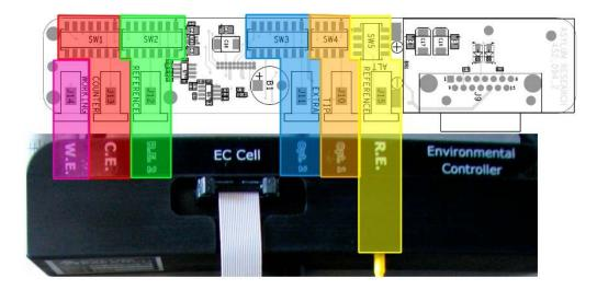
**Figure 24.13.:** Dip switches and circuit board seen from the bottom of the patch box. This graphic indicates the corresponding connector for each switch on the outside of the Junction Box.
