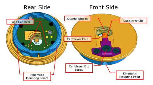
Figure 4.1.: Standard cantilever holder nomenclature
