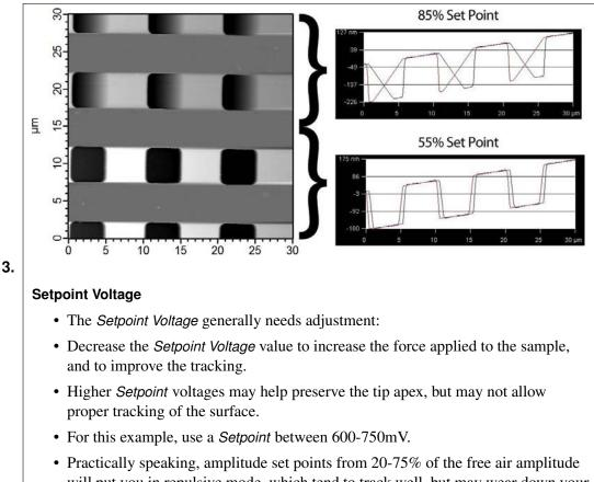
• Practically speaking, amplitude set points from 20-75% of the free all amplitude will put you in repulsive mode, which tend to track well, but may wear down your tip.
