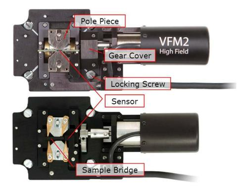
**Figure 25.10.:** Some of the basic components of the VFM defined. Also a side by side comparison of the samples stages of the VFM and the VFM2-Tesla. The original VFM can be distinguished by the lacking text on the motor cover, no gear cover, and no small sensor circuit board between the pole pieces.
