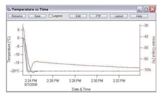
**Figure 20.6.:** The latter part of this graphs shows the heater power as the temperature ramps down to -20C. Note the steady increase in cooler power due to the body of the cooler heater warming up and the Peltier has to work harder to maintain the temperature setpoint.
