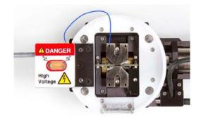
General sample mounting is described in Section 25.9 on page 387. Depending on your application you may need to make certain that the sample has (or does not have) a good electrical connection to the grounded pole pieces. We have supplied a few extra ground wires and pins in case you want to arrange for a wire directly to your sample.
