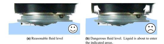
**Figure 7.2.:** Flooding of the cantilever holder can be a serious problem. Keep an eye on fluid levels, or better yet, image only with a membrane attached to the cantilever holder.
