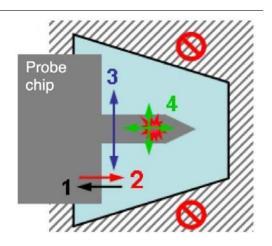
**3.** A successful positioning will result in a red spot on the IR card which looks split since its center is obscured by the cantilever. A slight movement of LDY away from the lever should reduce the SUM to near zero and make the spot on the IR card light up brightly again.
