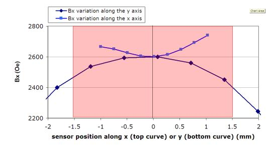
**Figure 25.8.:** Variation of the x component of the magnetic field along the x and y axes (with z=0). Pole faces were separated by ~3mm. x-axis data cannot extend the full 3mm range due to the sensor plastic enclosure hitting the pole faces. The pole faces are also 3mm wide andF so the red area indicates measurements taken with the sensor in the gap between the faces.
