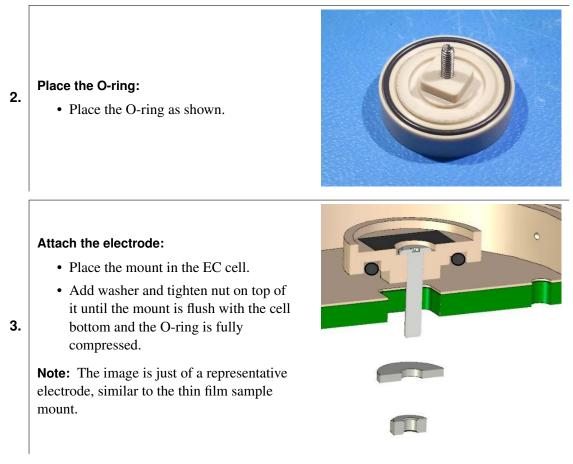
The nut makes contact with the circuit board which then automatically routes the connection to the junction box via the flat cable.
