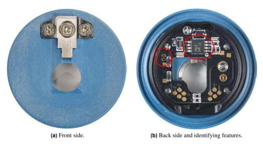
Figure 21.2.: Dual Gain ORCA Cantilever Holder.
