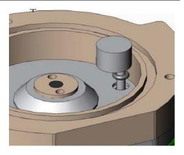
Note that with the second generation electrode, the O-ring groove varies in width so that the O-ring can be more easily removed. Only pry the O-ring loose with a soft toothpick and be careful not so scratch the soft graphite surface against which the O-ring must seal.
