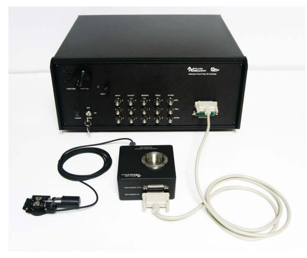
**Figure 25.2.:** TheVFM sample stage plugs into the 9-pin connector on the VFM controller box. This in turn plugs into the 25-pin expansion connector on the front of the MFP-3D controller. This photo shows the older MFP-3D controller. The newer ARC2 controller can be used as well.
