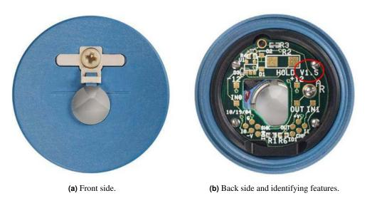
Figure 11.3.: PEEK Cantilever holder.
