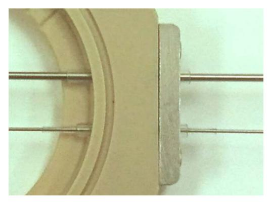
**Figure 14.7.:** Top: A piece o 230.006 tubing sleeved around a 1.0mm diameter wire. Bottom, a piece of 231.019 tubing sleeved around a piece of 231.028 tubing sleeved around a 0.4mm diameter wire.
