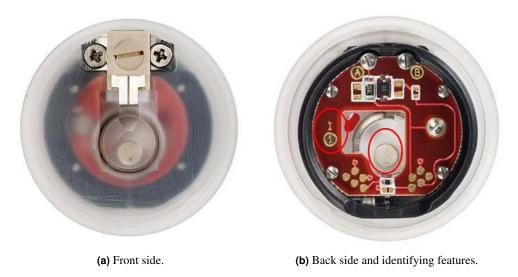
Figure 11.9.: iDrive Fluorescence Cantilever holder.
