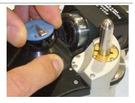
• Pulling or jiggling the cantilever holder should result in no motion.
