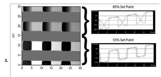
Setpoint Voltage The Setpoint Voltage generally needs adjustment:
