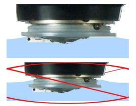
**Realigning the Laser Beam** Once the cantilever has been fully immersed in liquid, the SUM signal will disappear. This is because the optical path is different due to the change in the index of refraction. The light beam needs to be redirected to the lever to regain the signal.
