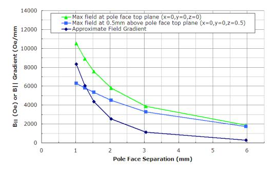
**Figure 25.7.:** Maximum field along the x-axis measured at the origin (sample in plane with pole face tops) and 0.5mm above (0.5mm thick sample resting on pole face tops). Also, the approximate field gradients at each point for Z=0.
