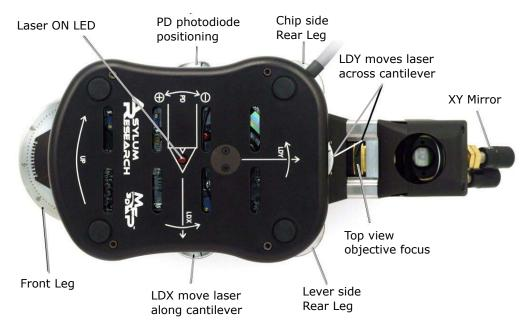
**Figure 2.3.:** Top view of the AFM head with named controls. Note the cantilever shape in the middle (same orientation as the real cantilever) and the LED at the tip of this lever. The red LED lights up when the laser is on (but not necessarily focused on the tip).
