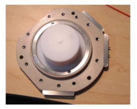
**4.** If you are only interested in maintaining one humidity value, you can plug any remaining open ports, place the humidity cell on the scanner, fill the reservoir with the desired salt solution, place your sample, and skip ahead to Section 19.7.2.3 on page 254. If you want to have the option of changing humidity during an experiment, then please keep following the next steps.
