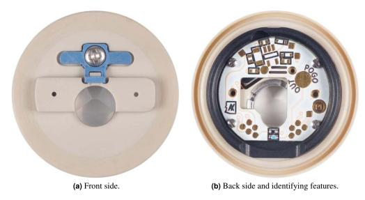
Figure 11.6.: MicroFlow cantilever holder
