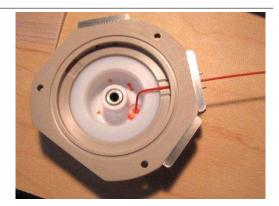
**6.** Move the cell over to the AFM and place your sample on it. You can start out by filling up the reservoir without the AFM head in place. If needed, you can pull out the fluid, and put in a different fluid all while the AFM is operating.
