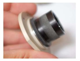
**Note** The initial threading process should be smooth. If not, you may have crossed threads - this can cause damage the peek cell body.
