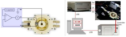
(a) Basic connection to be made to the idealized potentiostat, shown diagrammatically.
