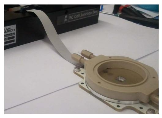
Figure 24.19.: EC Cell assembled with the heater stage installed.
