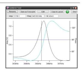
**Note** Cleaner tunes can be obtained by blowing the cantilever holder with compressed air prior to loading cantilever to get rid of any left over silicon/glass debris.
