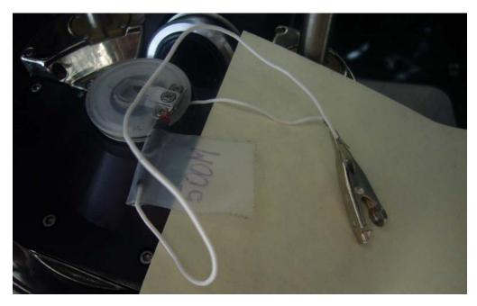
Figure 21.4.: Connect the test resistor in between the bias wire and the probe clip as shown
