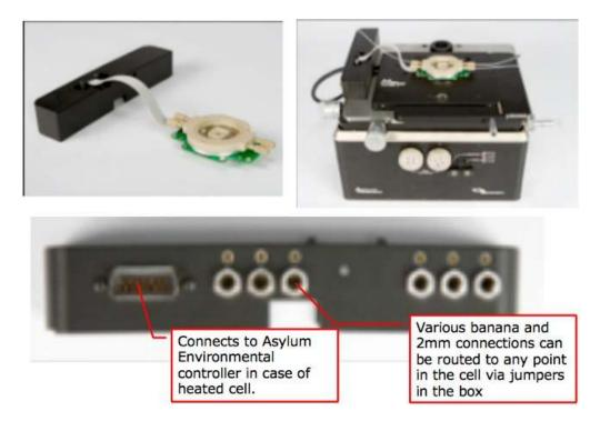
**Figure 24.11.:** The EC Cell plugged into the Junction Box, and the Junction Box and EC Cell on the MFP-3D AFM. Finally, a close-up of the Junction Box Connections.
