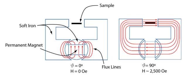
**Figure 25.1.:** How it works: A rare earth permanent magnet is at the heart of the VFM. The strength and sign of the magnetic field applied to the sample depends on the rotation angle of the magnet. When the magnet is at 0° or 180°, the magnetic flux is shunted away from the sample by the soft iron armature and pole pieces. As the magnet rotates, more and more flux is channeled instead through the sample. At 90° and 270°, the field magnitude is maximized.
