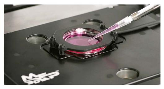
**Figure 23.5.:** Picture of Petri dish with clamp sitting on the scanner. Open access to the sample when the head has been removed.
