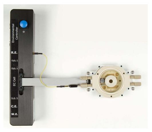
Figure 24.1.: EC Cell Fully Assembled
