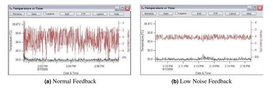
Figure 20.7.: Controlling Temperature near room temperature with and without the low nose option.
