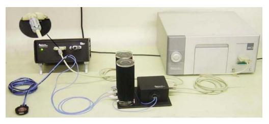
Figure 20.2.: Full setup with coolant pump, for -20 to +120C operation.
