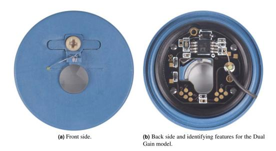
Figure 11.7.: PEEK ORCA Cantilever holder (Dual Gain).
