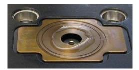
**NOTE:** Be careful not to use an excessive amount of immersion oil. You SHOULD NOT get oil on the XY scanner as it may flow inside the scanner and cause damage.
