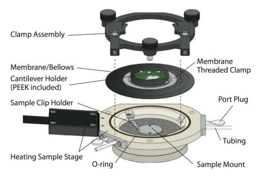
Figure 18.2.: A nice overview of the polymer heater and its parts.
