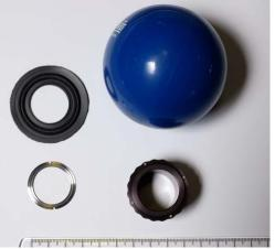
**NOTE:** Old versions of retaining ring did not have an O-ring groove. Make sure you are using the ring which does indeed have the O-ring groove.
