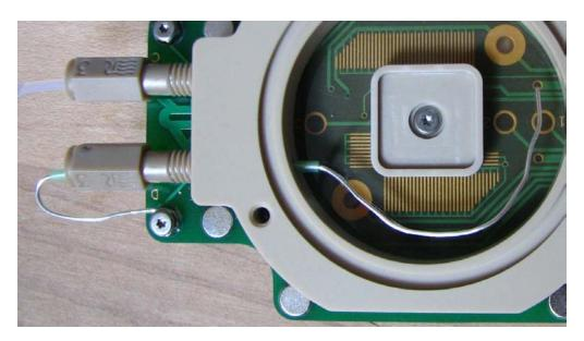
**Figure 24.8.:** A silver wire passed through a fluid port fitting using a green Teflon sleeve. Wire is connected to screw terminal D.
