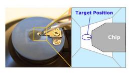
**Note** The quartz window is resilient to scratching from tweezers, so do not be paranoid.
