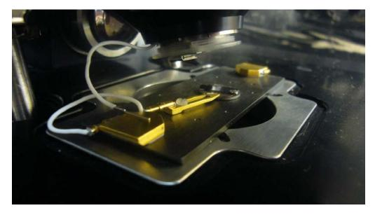
for an example a mounted sample with the jumper wire attached.
