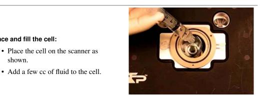
2. Prepare your cantilever for fluid imaging. Wet the cantilever with a bit of fluid as described in Step 2 on page 69.
