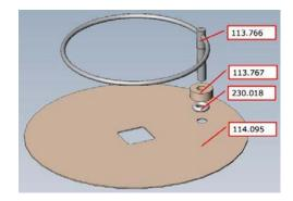
This electrode is not standard equipment - it can be bought from Asylum Research for an extra charge, due to the high price of platinum. Please inquire about assembly number 939.020 which will include all the parts described in this section.
