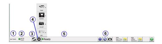
Along the bottom of the screen. Icon controls relate to the status of connected instrument components. The low level software version is also displayed.
