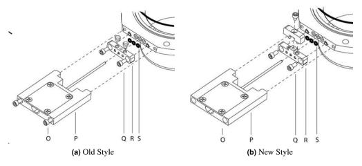
Figure 17.4.: Bioheater heating element clamping mechanisms.
