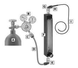
**Figure 14.4.:** Typical gas flow system. M denotes McMaster Carr part number, A indicates Asylum Research Part Number.
