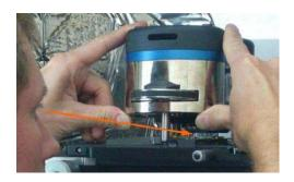
**Tip** A white piece of paper taped to the back of the hood makes for a good back-ground against which to see the cantilever holder.
