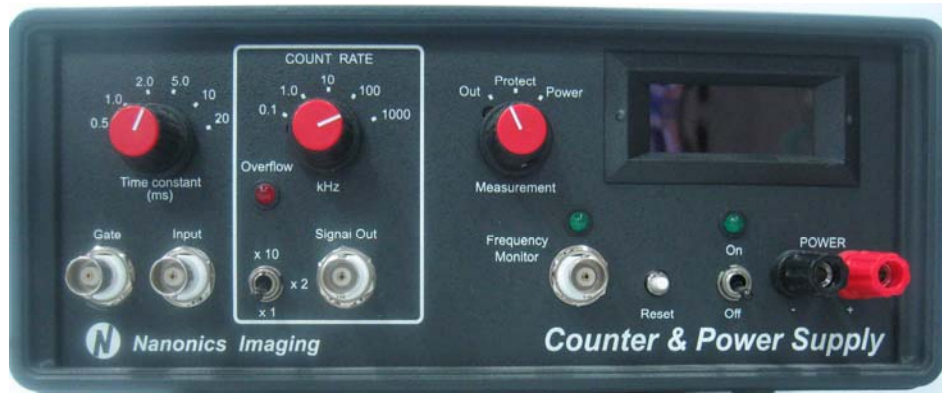
Figure 27: APD Counter and Power Supply
