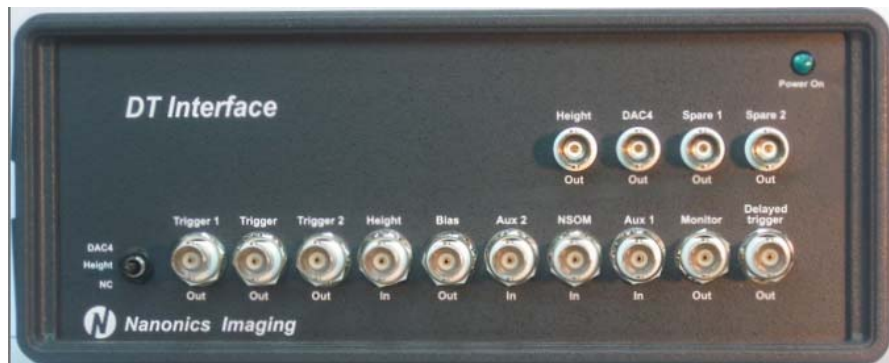
Figure 19: DT Front Panel
