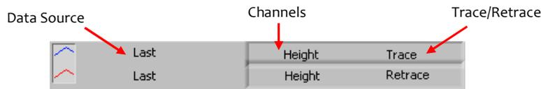
Figure 5: Changing the scope monitor display
