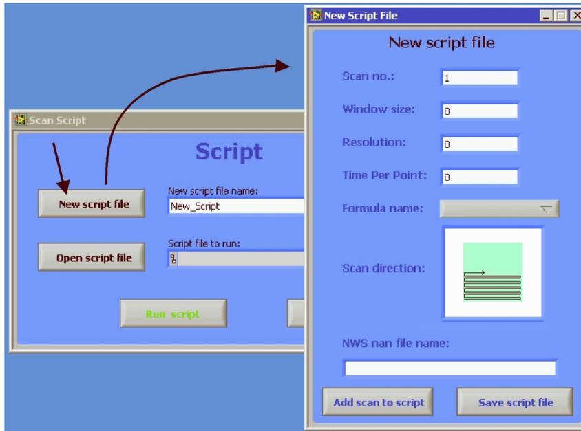
3. In this window, you can choose the window size, resolution, time per point, formula, scan direction and the NWS nan file name for each scan. The NWS nan file name can be automatically set as Scan\_%no.%\_Window\_size\_%no.%\_nan in the "Script Scans" directory, for each scan respectively.
