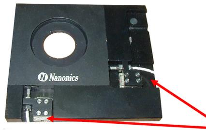
Use a screwdriver to move the sensors until the output voltage is about 5 V. This ensures that the sensors are at the zero position.
