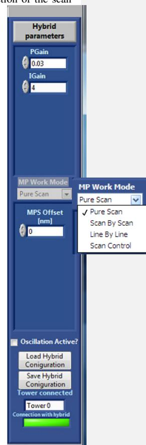
7. **Load Hybrid Configuration/Save Hybrid configuration buttons.** Possibility to load previously saved Hybrid parameters or to save it
