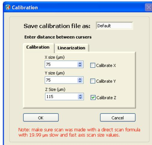
*Figure 14: The calibration window*
