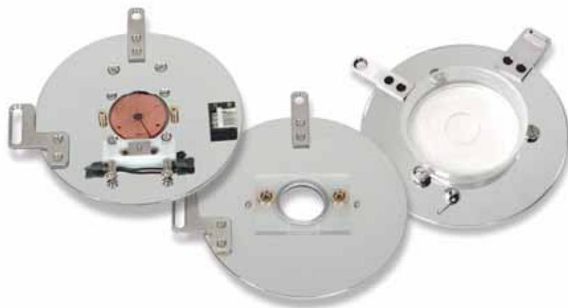
**Figure 16** Three sample plates: MAC Mode, liquid cell, and Petri dish
