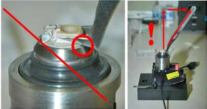
**Figure 35** Do not use tweezers to remove a nose assembly. Doing so can place damaging lateral forces on the scanner.
