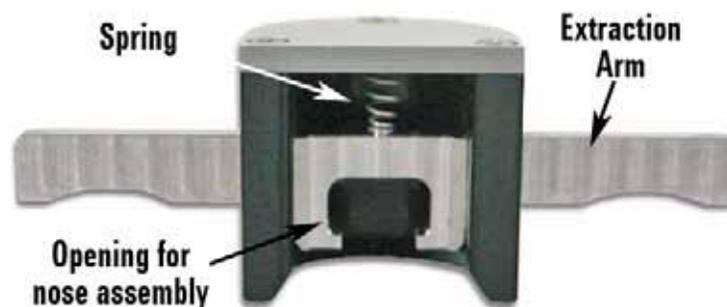
**Figure 33** Nose assembly removal tool
