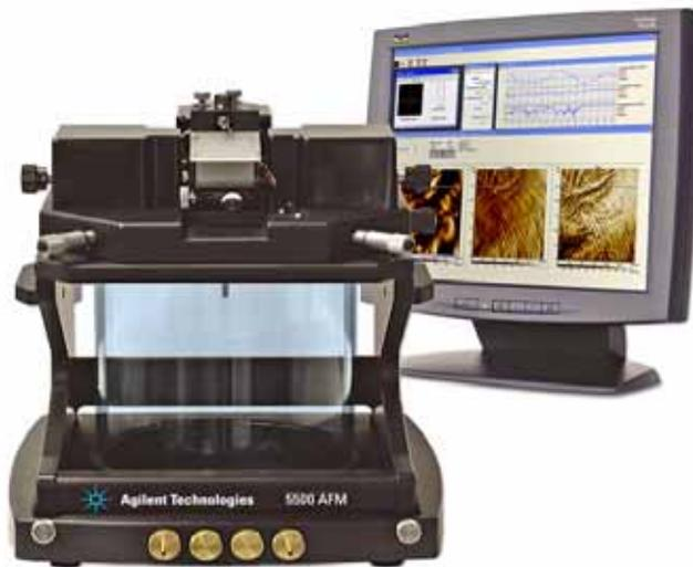
**Figure 1** The Agilent 5500 SPM microscope, shown with optional environmental chamber
