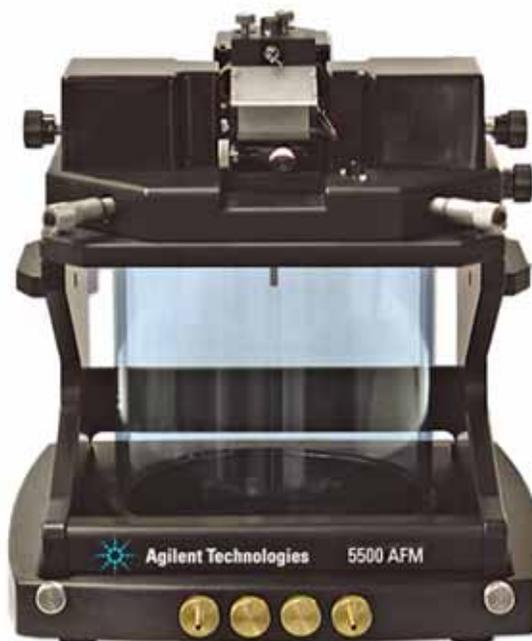
**Figure 141** Environmental chamber on microscope
