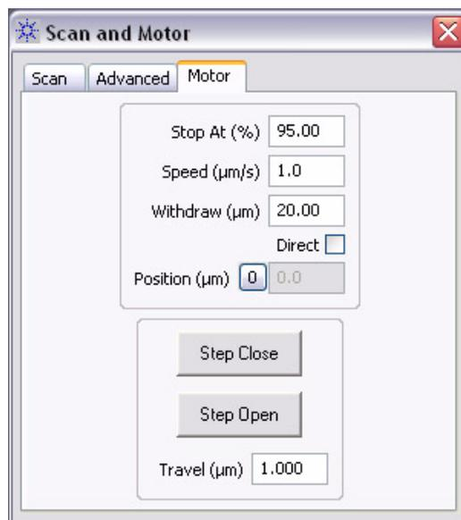
**Figure 73** Set the Stop At value in the Scan and Motor window
