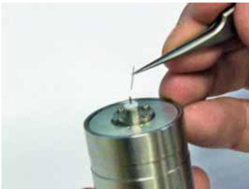
**Figure 80** Inserting STM tip wire in scanner
