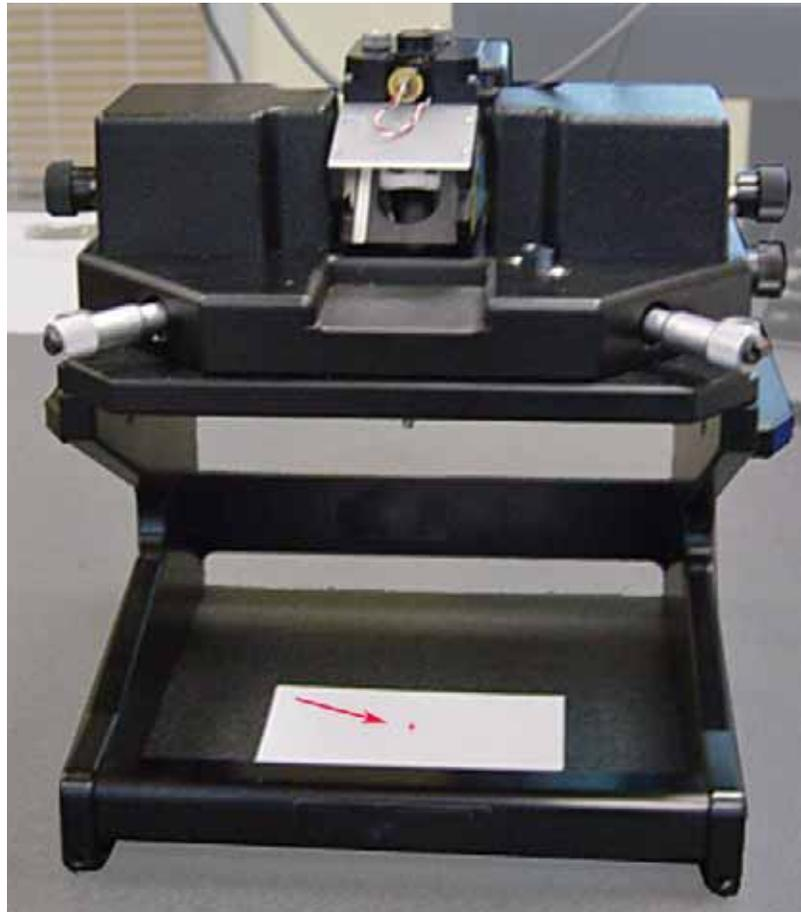
**Figure 46** Aligning laser spot over white paper.
