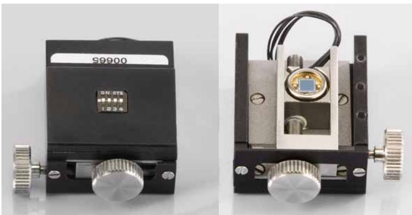
**Figure 15** Detector assembly, top and bottom views
