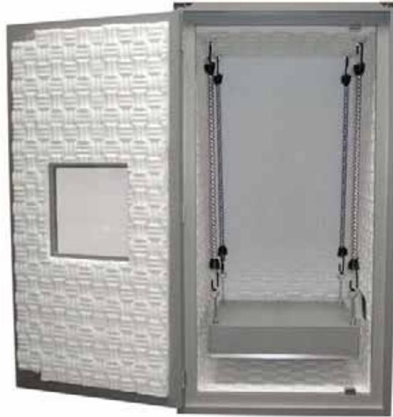
**Figure 23** Vibration isolation chamber
