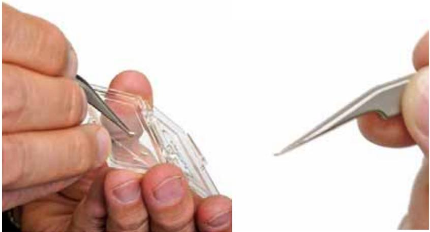
**Figure 38** Holding the tweezers as shown, remove a probe from the protective case
