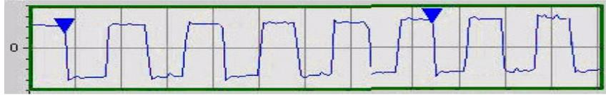
**Figure 94** Horizontal cross-section tool used to check non-linearity. Two sets of cursors are shown.
