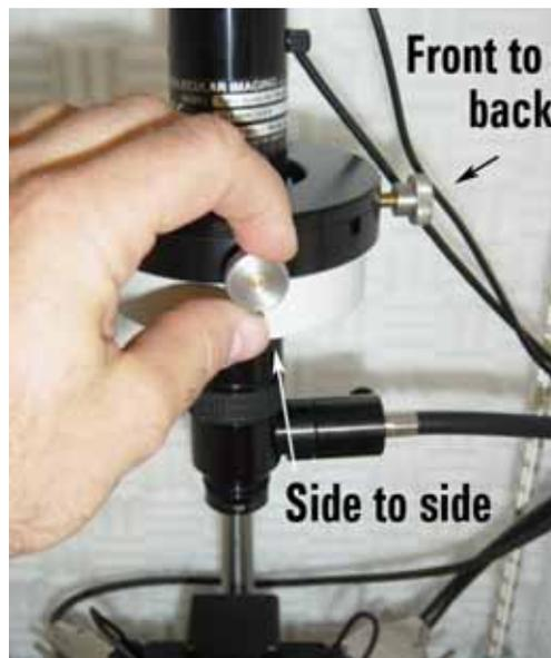
**Figure 60** Adjusting lateral position of the video system
