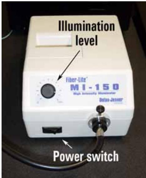
**Figure 58** Turn on the illuminator and adjust intensity
