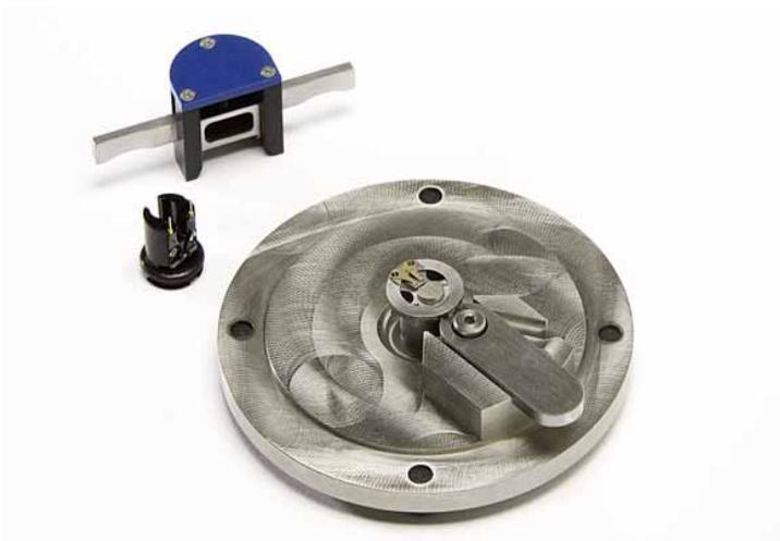
**Figure 13** Two-piece nose cone with removal tool and assembly jig
