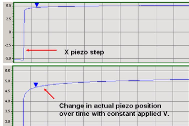
**Figure 91** Scanner creep
