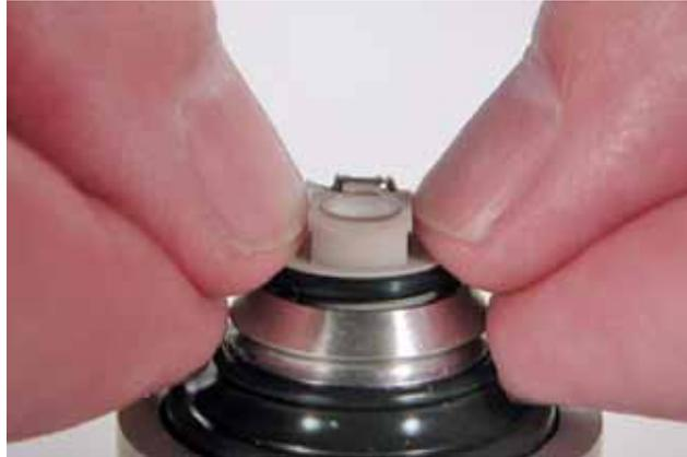
**Figure 32** Applying even, vertical pressure at the edges to insert the nose assembly.
