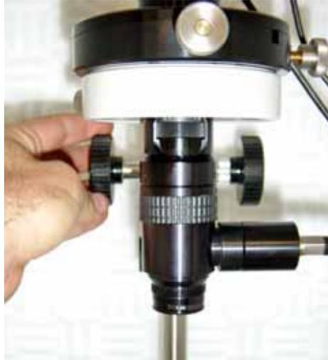
**Figure 59** Adjusting the z-position
