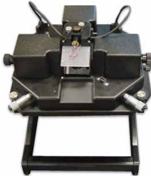
**Figure 11** 5500 SPM microscope on support stand
