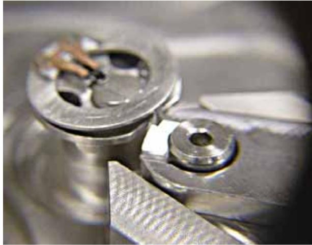
**Figure 43** Move the lever to open the nose assembly disk.
