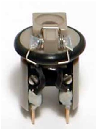
**Figure 70** AAC Mode nose assembly
