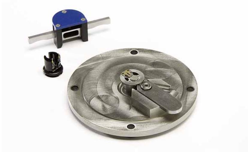
**Figure 40** Two-piece nose assembly, removal tool and assembly jig. The nose assembly disk is shown on the jig; the body is shown to its left.
