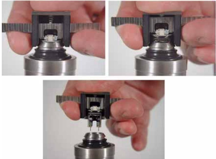
**Figure 34** Using the nose assembly removal tool
