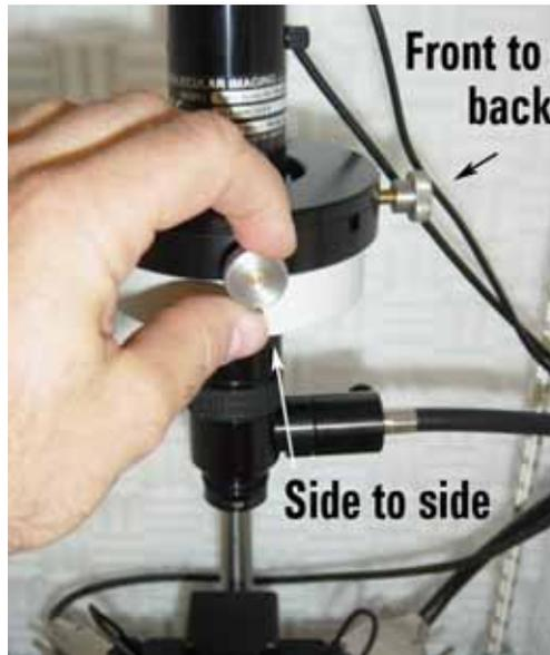
**Figure 60** Adjusting lateral position of the video system
