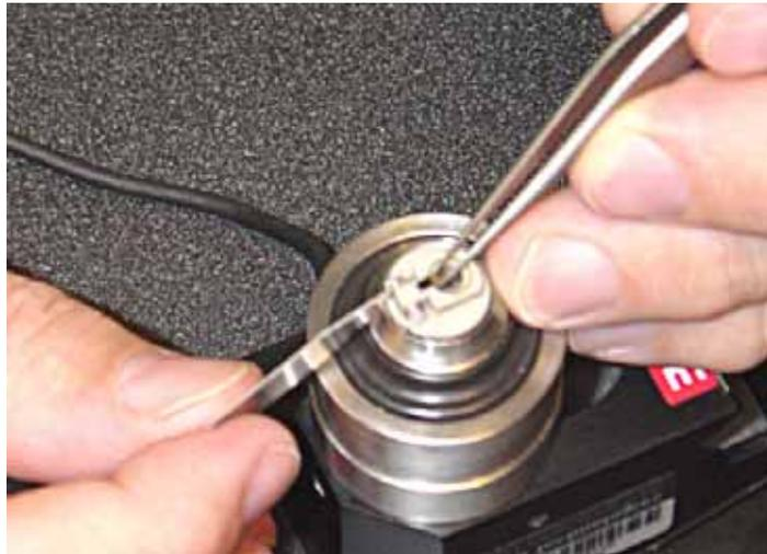
**Figure 39** Hold back the retaining spring while placing the probe
