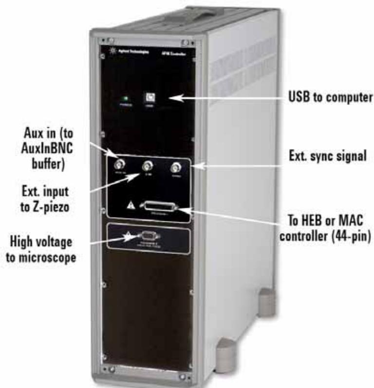
**Figure 22** AFM Controller (Model 3000)
