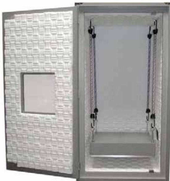
**Figure 23** Vibration isolation chamber
