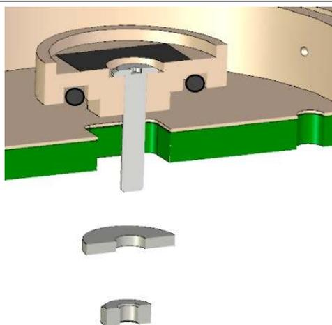
The nut makes contact with the circuit board which then automatically routes the connection to the junction box via the flat cable.
