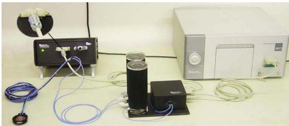
**Figure 20.2.:** Full setup with coolant pump, for -20 to +120C operation.
