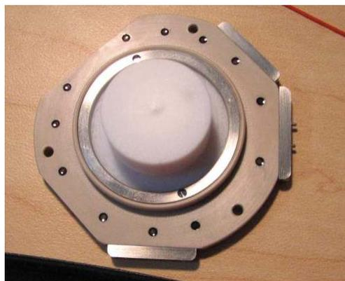
4. If you are only interested in maintaining one humidity value, you can plug any remaining open ports, place the humidity cell on the scanner, fill the reservoir with the desired salt solution, place your sample, and skip ahead to [Section 19.7.2.3 on page 254](#). If you want to have the option of changing humidity during an experiment, then please keep following the next steps.
