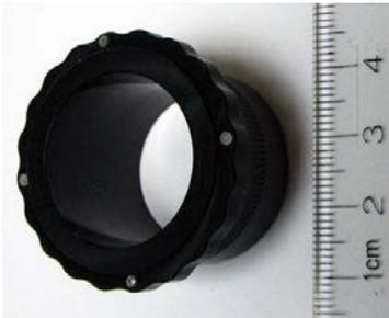
A black, circular, multi-ported spanner wrench assembly is shown next to a ruler for scale. The ruler indicates the diameter is approximately 3.5 cm.                                   |
