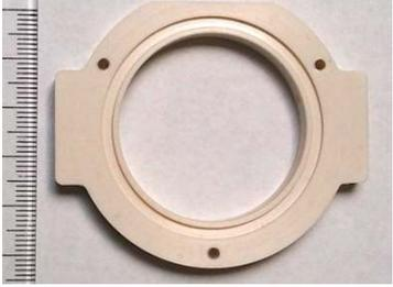
A tan-colored EC Cell Body, PPS, showing a circular opening and four mounting holes. A ruler is visible on the left side for scale.                              |
