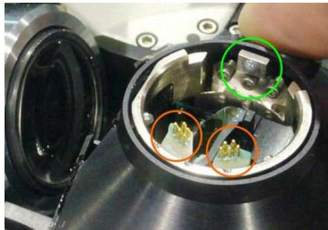
**Inspect mounting of the cantilever holder:**
