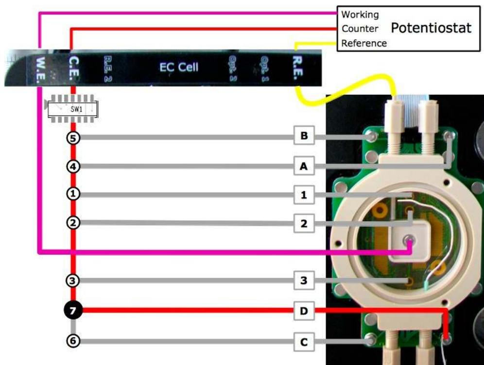
**Figure 24.15.:** Dip Switch 1, position 7 is set to ON so that corner terminal D (Connected to a metal wire counter electrode) is routed to the C.E. connector on the Junction Box.
