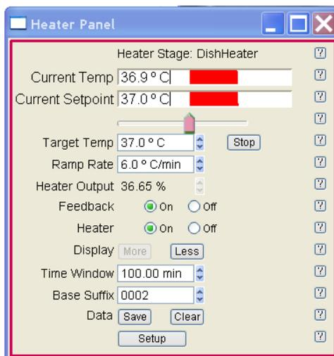
**Figure 23.2.:** Heater Panel window
