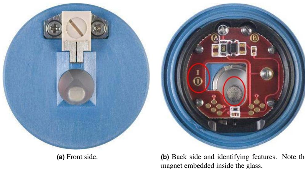
**Figure 11.8.:** iDrive Cantilever holder.
