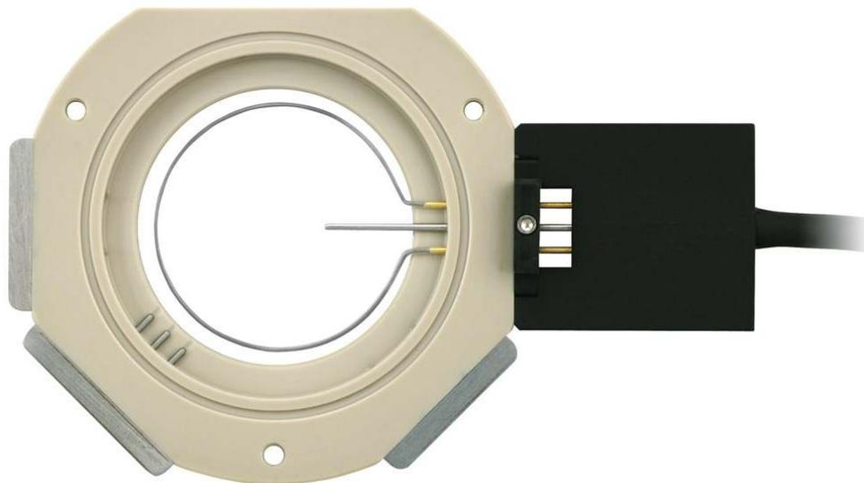
Figure 17.1.: Top View of assembled bioheater.
