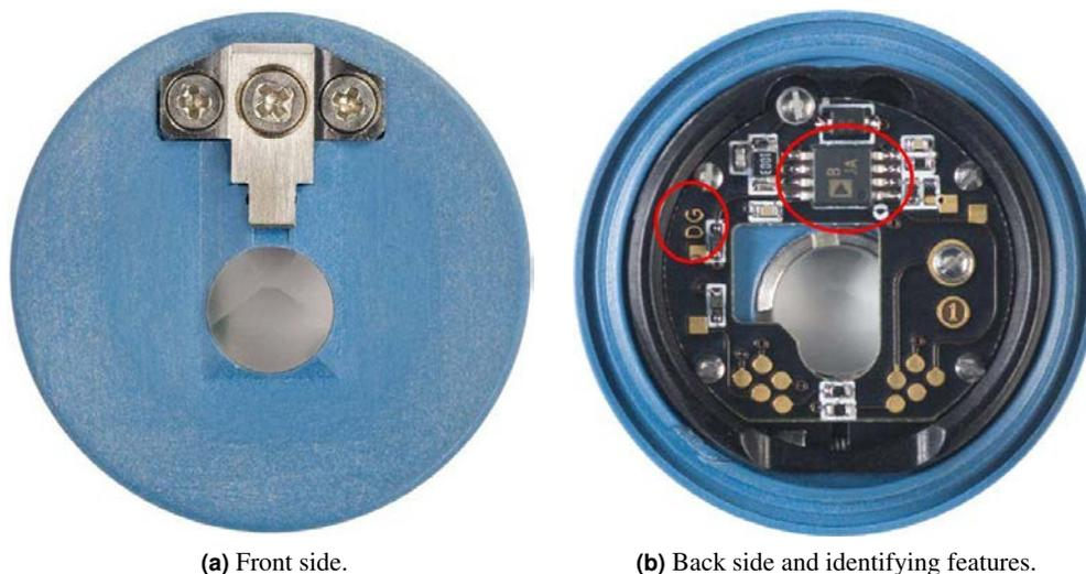
Figure 21.2.: Dual Gain ORCA Cantilever Holder.
