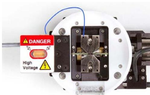
General sample mounting is described in [Section 25.9 on page 387](#). Depending on your application you may need to make certain that the sample has (or does not have) a good electrical connection to the grounded pole pieces. We have supplied a few extra ground wires and pins in case you want to arrange for a wire directly to your sample.
