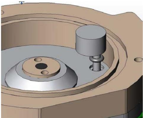
Note that with the second generation electrode, the O-ring groove varies in width so that the O-ring can be more easily removed. Only pry the O-ring loose with a soft toothpick and be careful not to scratch the soft graphite surface against which the O-ring must seal.
