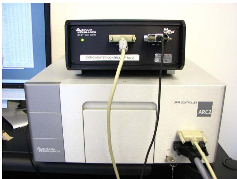
**Figure 16.2.:** Environmental Controller connected to an ARC2 AFM Controller with a DB25 cable with interrupted shield (see gray sleeve close to one end). A temperature stage is plugged into the Environmental Controller.
