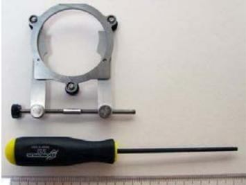
A metal membrane clamp assembly is shown next to a ruler and a screwdriver for scale. The assembly consists of a circular ring with two clamping points and a central screw mechanism. |
