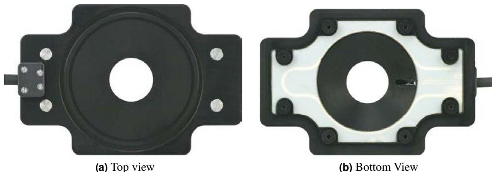
**Figure 23.1.:** Top (left) and side (right) views of the Petri Dish Holder. The photo on the right also shows the magnetic clamp holding down a glass bottom Petri dish.
