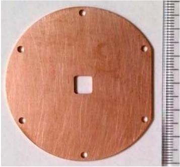
A circular copper film counter electrode with a central square hole and four small holes around the perimeter. A ruler is visible on the right side for scale.     |
