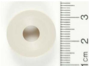
A white, shallow, circular nut with a central hole. A ruler to the right shows a scale from 0 to 3 cm.             |
