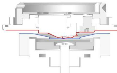
(b) Cantilever holder clearance when using the thin film sample mount. Space is tight. In reality the nut which seals against the sample bends a bit making the gently sloped sides closer to horizontal, creating a bit more space than what is shown in this CAD drawing.
