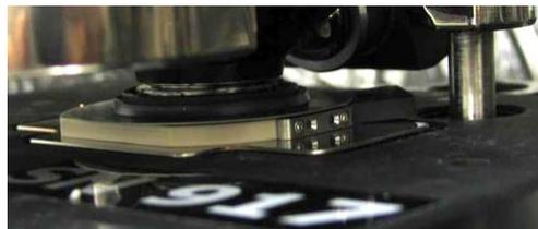
**Caution!** **DO NOT** suddenly lift up the AFM head. The combination of suction and magnetic clamping will likely cause the cell to fly up, which will break the probe and make a salty mess all over your AFM. **FIRST break the seal** by prying a flat tool between the cell body and the membrane. **ONLY THEN lift the head.**
