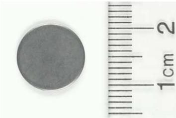
A circular, grey AFM disc is shown next to a ruler for scale. The ruler indicates the diameter is 12 mm.                                            |
