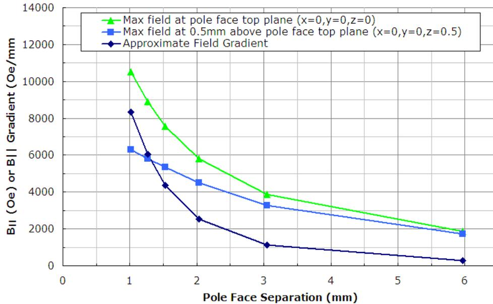
**Figure 25.7.:** Maximum field along the x-axis measured at the origin (sample in plane with pole face tops) and 0.5mm above (0.5mm thick sample resting on pole face tops). Also, the approximate field gradients at each point for  $Z=0$ .
