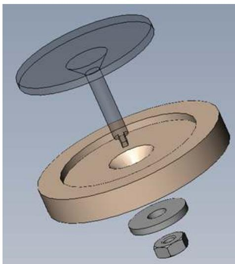
**Figure 24.23.:** Experimental Parafilm sample mount 939.018.
