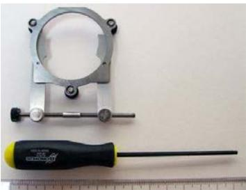
A metal membrane clamp assembly is shown with a screwdriver and a ruler for scale. The ruler indicates the diameter is approximately 2.5 cm.          |
