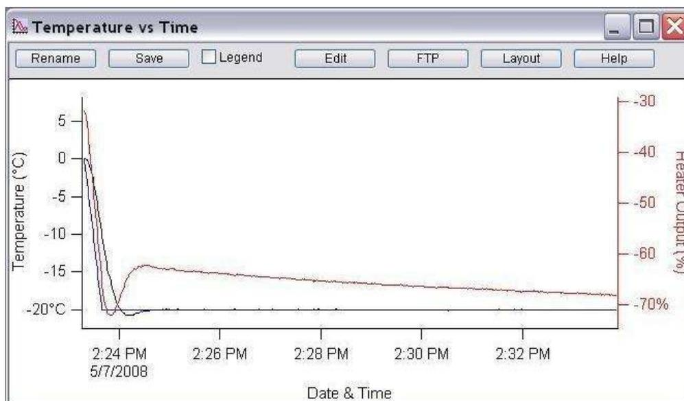
**Figure 20.6.:** The latter part of this graphs shows the heater power as the temperature ramps down to -20C. Note the steady increase in cooler power due to the body of the cooler heater warming up and the Peltier has to work harder to maintain the temperature setpoint.
