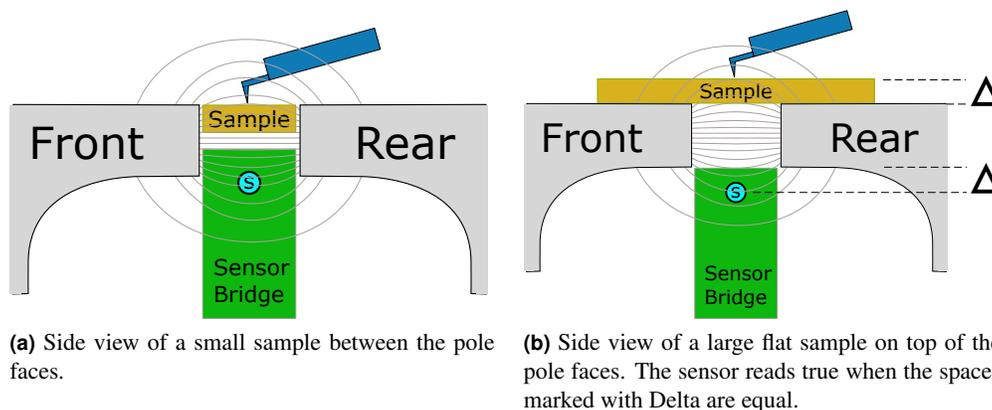
**Figure 25.9.:** Side views showing a small sample mounted between the pole faces with its top surface flush with the top of the pole faces. This allows for the maximum field. In sub figure B, a larger flat sample sitting on top of the pole faces is shown. The max field is less and the distance from the top edge of the pole faces to the top of the sample needs to equal the distance from the bottom edge of the pole faces to the sensor (The two Delta spaces).
