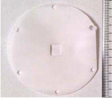
A circular white PTFE film counter electrode with a central square hole and four small holes around the perimeter. A ruler is visible on the right side for scale. |
