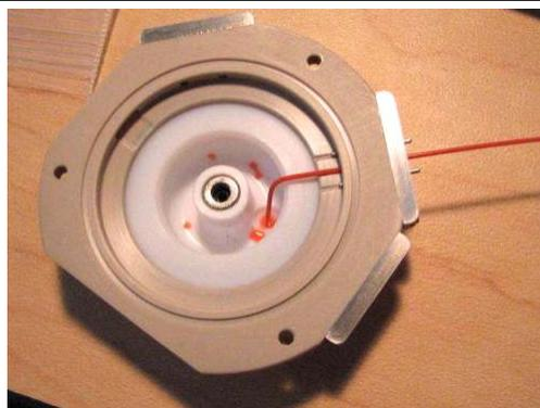
6. Move the the cell over to the AFM and place your sample on it. You can start out by filling up the reservoir without the AFM head in place. If needed, you can pull out the fluid, and put in a different fluid all while the AFM is operating.
