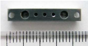
A rectangular stainless steel bar with three circular ports, shown next to a ruler for scale.                            |
