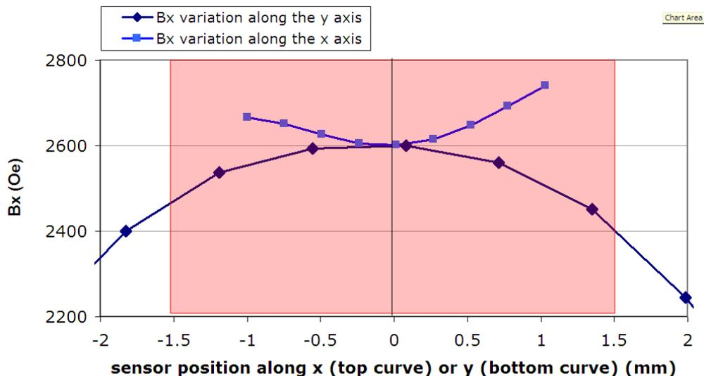
**Figure 25.8.:** Variation of the x component of the magnetic field along the x and y axes (with  $z=0$ ). Pole faces were separated by  $\sim 3$ mm. x-axis data cannot extend the full 3mm range due to the sensor plastic enclosure hitting the pole faces. The pole faces are also 3mm wide and so the red area indicates measurements taken with the sensor in the gap between the faces.
