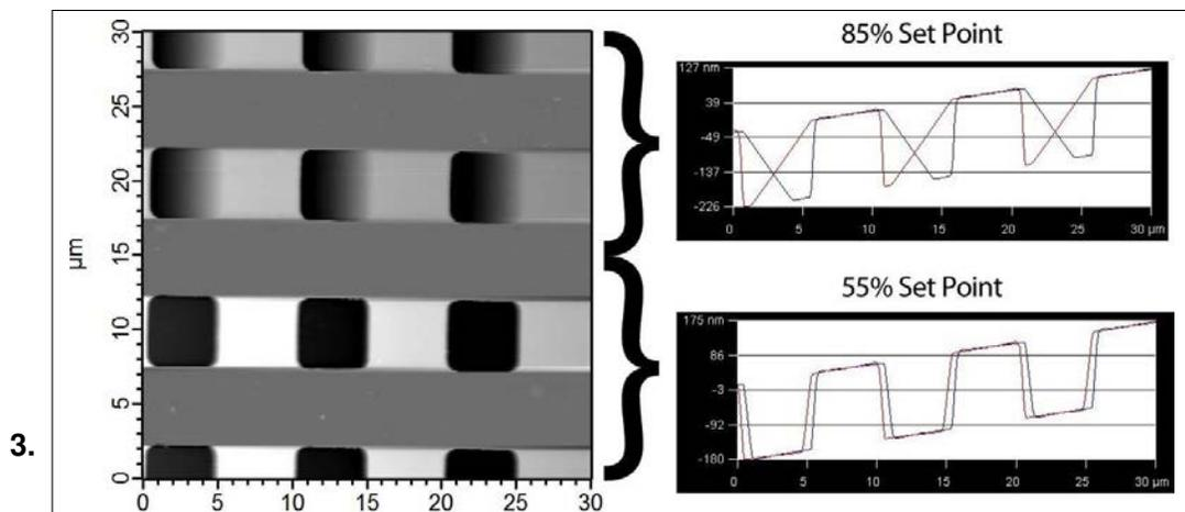
**Setpoint Voltage** The *Setpoint Voltage* generally needs adjustment:
