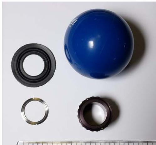
**NOTE:** Old versions of retaining ring did not have an O-ring groove. Make sure you are using the ring which does indeed have the O-ring groove.
