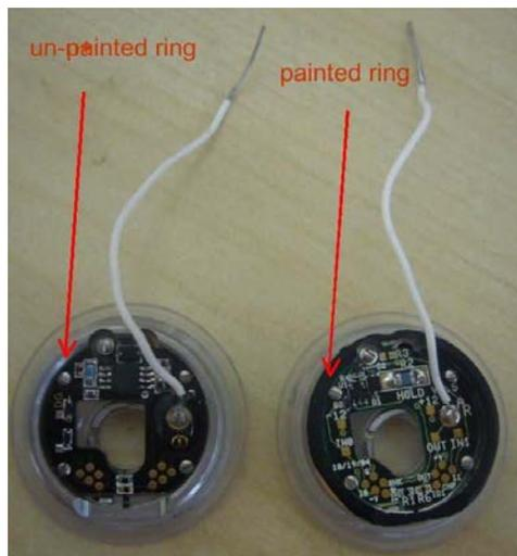
**Figure 21.3.:** For ORCA holders without the painted ring, please use caution in loading them into the head, as the metal ring can short the op-amp.
