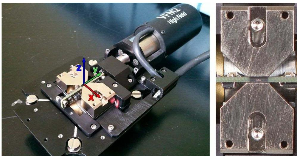
**Figure 25.4.:** Coordinate Axes defined and the field orientation. Positive sensor values are defined as B field components along the positive X-axis. To the right, a close up view of the preferred origin for imaging, which lies directly over the field sensor, highlighted as a tiny white line between the pole faces.
