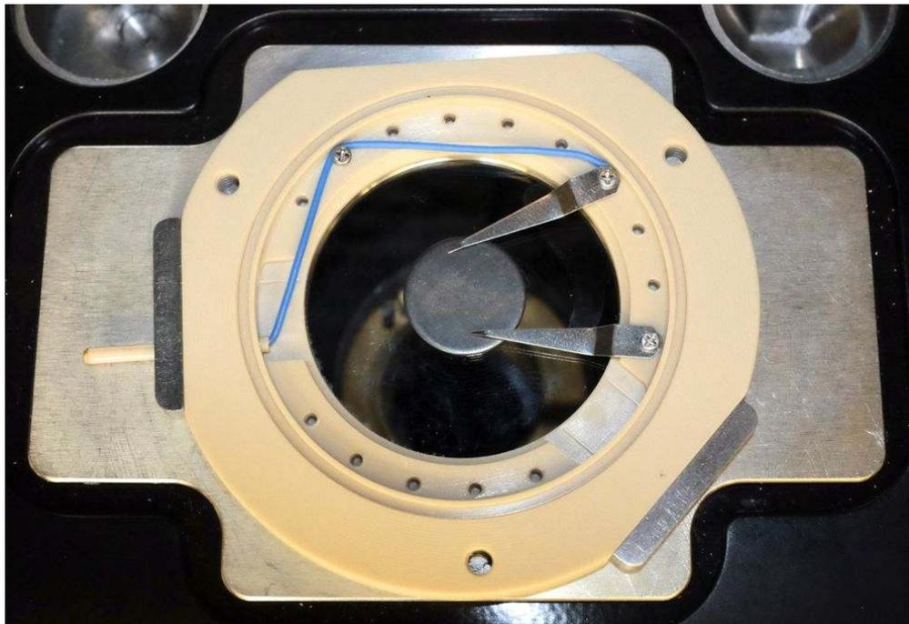
Figure 15.1.: The electrical closed cell in a typical configuration.
