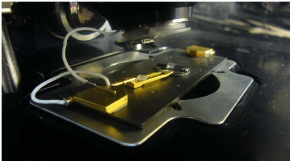
**Figure 21.5.:** Connect the bias wire that drops from the cantilever holder down to the magnet on the ORCA sample holder magnet as shown.
