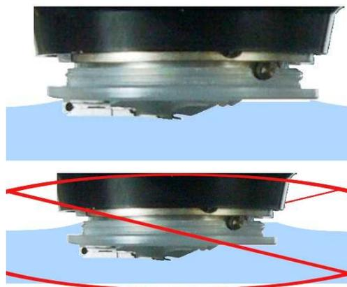
**Realigning the Laser Beam** Once the cantilever has been fully immersed in liquid, the SUM signal will disappear. This is because the optical path is different due to the change in the index of refraction. The light beam needs to be redirected to the lever to regain the signal.
