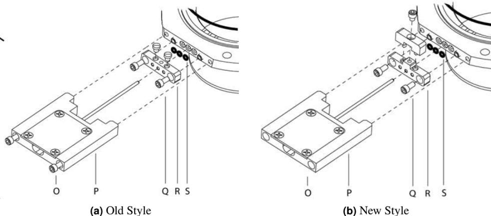
Figure 17.4.: Bioheater heating element clamping mechanisms.
