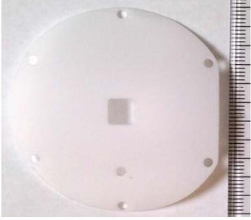
A circular white PTFE film counter electrode with a central square hole and one larger hole on the left side. A ruler is visible on the right side for scale.     |
