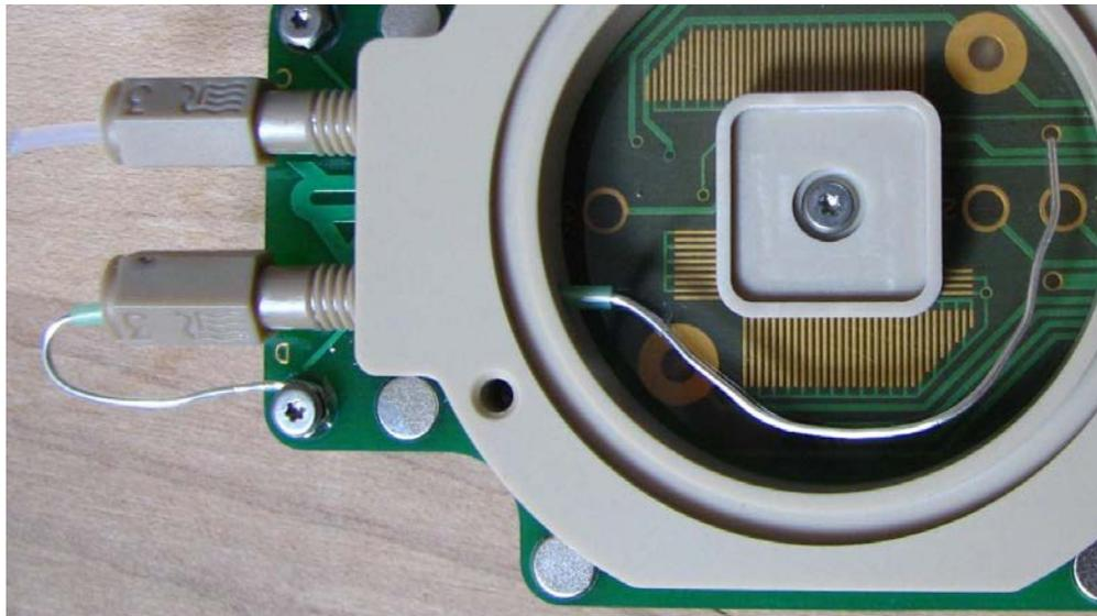
**Figure 24.8.:** A silver wire passed through a fluid port fitting using a green Teflon sleeve. Wire is connected to screw terminal D.
