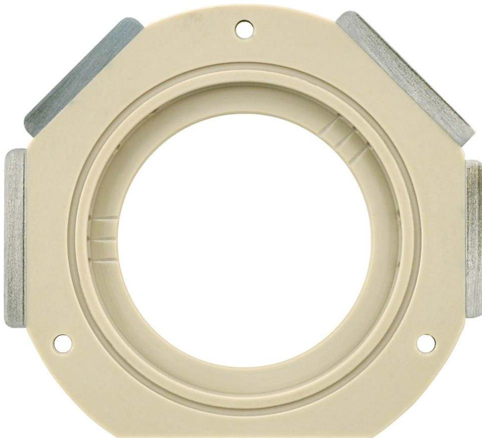
**Figure 14.1.:** Top view of the Closed Fluid Cell Body with port clamps installed.
