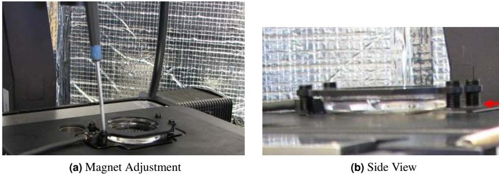
**Figure 22.3.:** Left: Adjusting the clamp screw depending on the height of the Petri dish. Right: Side view of the clamp on a low profile Petri dish showing a 1-2mm space between the magnet and the Petri Heater plate (red arrow)
