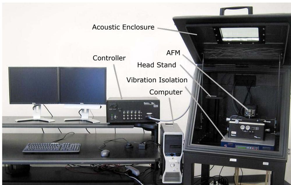
**Figure 2.1.:** Ideally the MFP-3D AFM with Stand Alone Base is set up as shown, with the controller and computer on one table and the AFM inside an acoustic enclosure. Note that newer systems operate with the ARC2 controller (see ?? on page ??).
