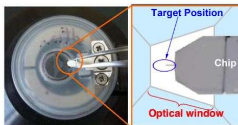
**Note** The cantilever holder was designed to be resilient, so do not worry about scratching it with tweezers.
