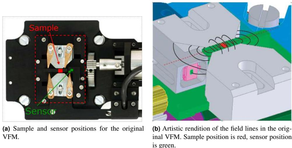
**Figure 25.11.:** The original VFM had the sensor positioned far away from the sample.
