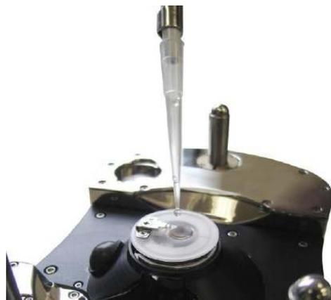
**Note** This step is optional, but highly recommended since it reduces the risk of creating air bubbles on the cantilever, and fills the space between the substrate and the bottom of the cantilever holder with liquid.
