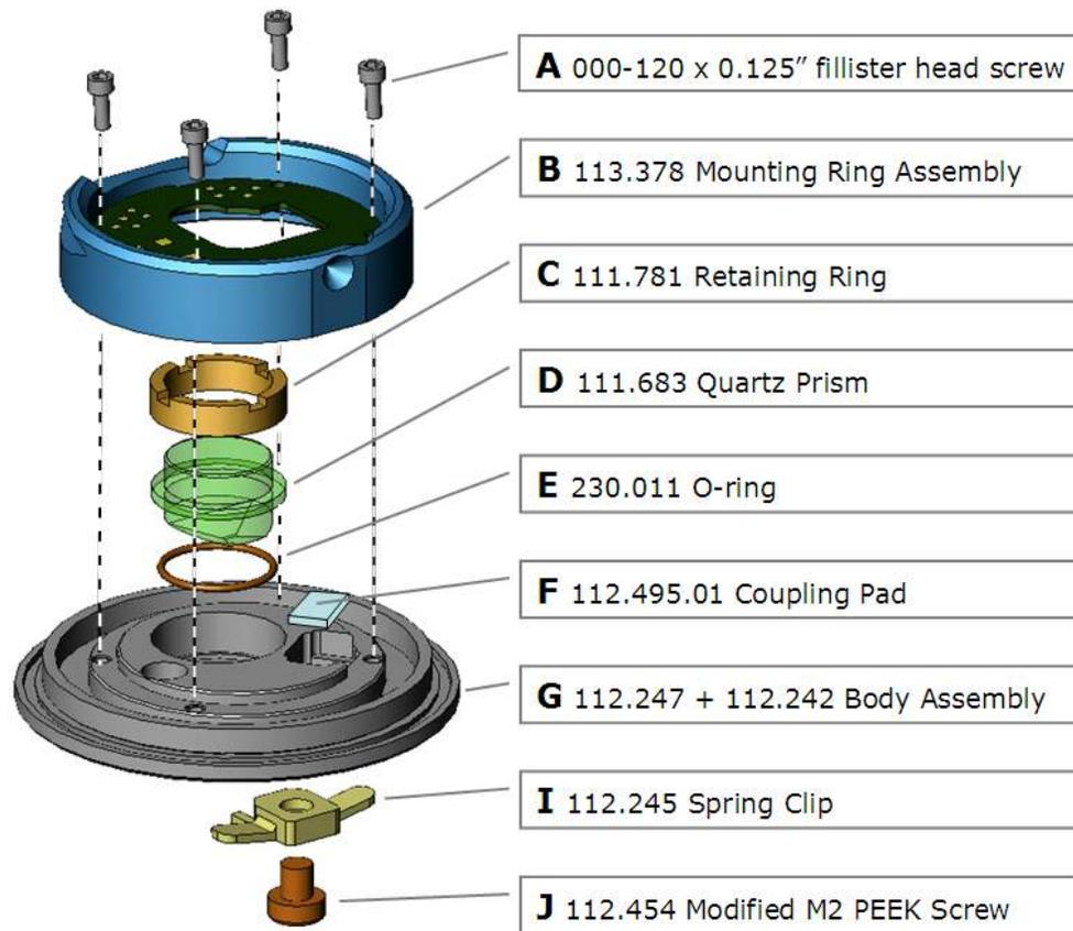
Figure 11.4.: PEEK Cantilever Holder Exploded.
