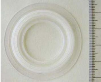
A clear, circular, closed-cell bellows component, shown next to a ruler for scale.    |
