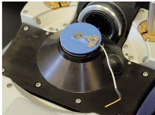
8. Since it is likely you will be operating the cell in a fully sealed configuration, attach the membrane to the cantilever holder as shown in [Section 13.4.3 on page 153](#). Still, before operating in a sealed configuration, we recommend you try to engage on a test sample with the cell open. Make sure that the image looks good and that no clips are rubbing against the cantilever holder. Read ahead a few steps and familiarize yourself with the process.
