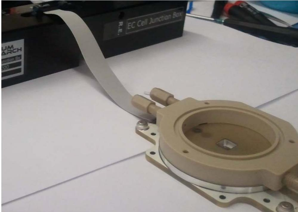
Figure 24.19.: EC Cell assembled with the heater stage installed.
