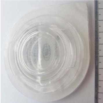
A clear, circular petri dish with a thin glass bottom, shown next to a ruler for scale. |
