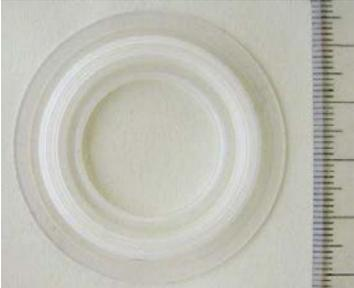
A white, circular, closed cell bellows component with a central hole, shown next to a ruler for scale.                  |
