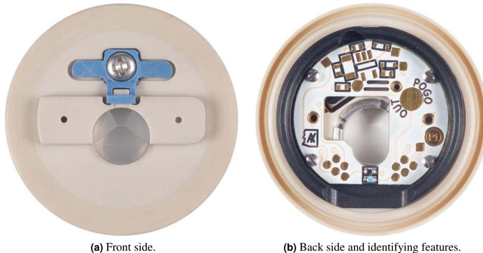
**Figure 11.6.:** MicroFlow cantilever holder
