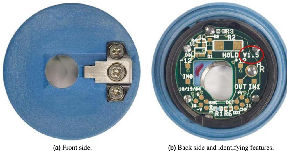
**Figure 11.1.:** Standard Cantilever holder.
