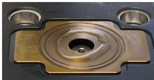
**NOTE:** Be careful not to use an excessive amount of immersion oil. You **SHOULD NOT** get oil on the XY scanner as it may flow inside the scanner and cause damage.
