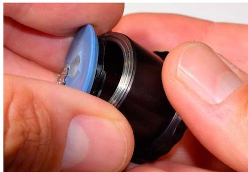
**Note** If there is any resistance, do not apply more force. Back off and turn the wrench a full turn counter clockwise to make sure ring seats properly onto the threads. This will give you a feel for the process and you may skip this step in the future.
