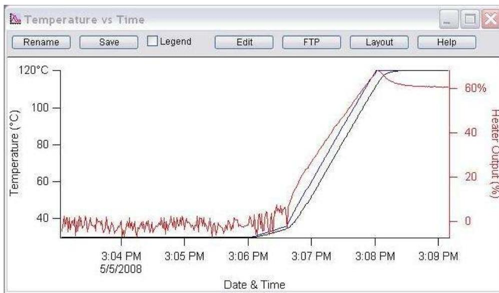
**Figure 20.5.:** The latter part of this graphs shows the heater power as the temperature ramps up to 120C.
