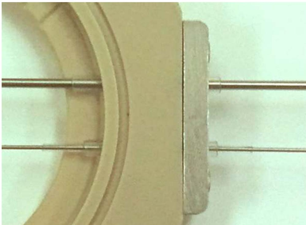
**Figure 14.7.:** Top: A piece of 230.006 tubing sleeved around a 1.0mm diameter wire. Bottom, a piece of 231.019 tubing sleeved around a piece of 231.028 tubing sleeved around a 0.4mm diameter wire.
