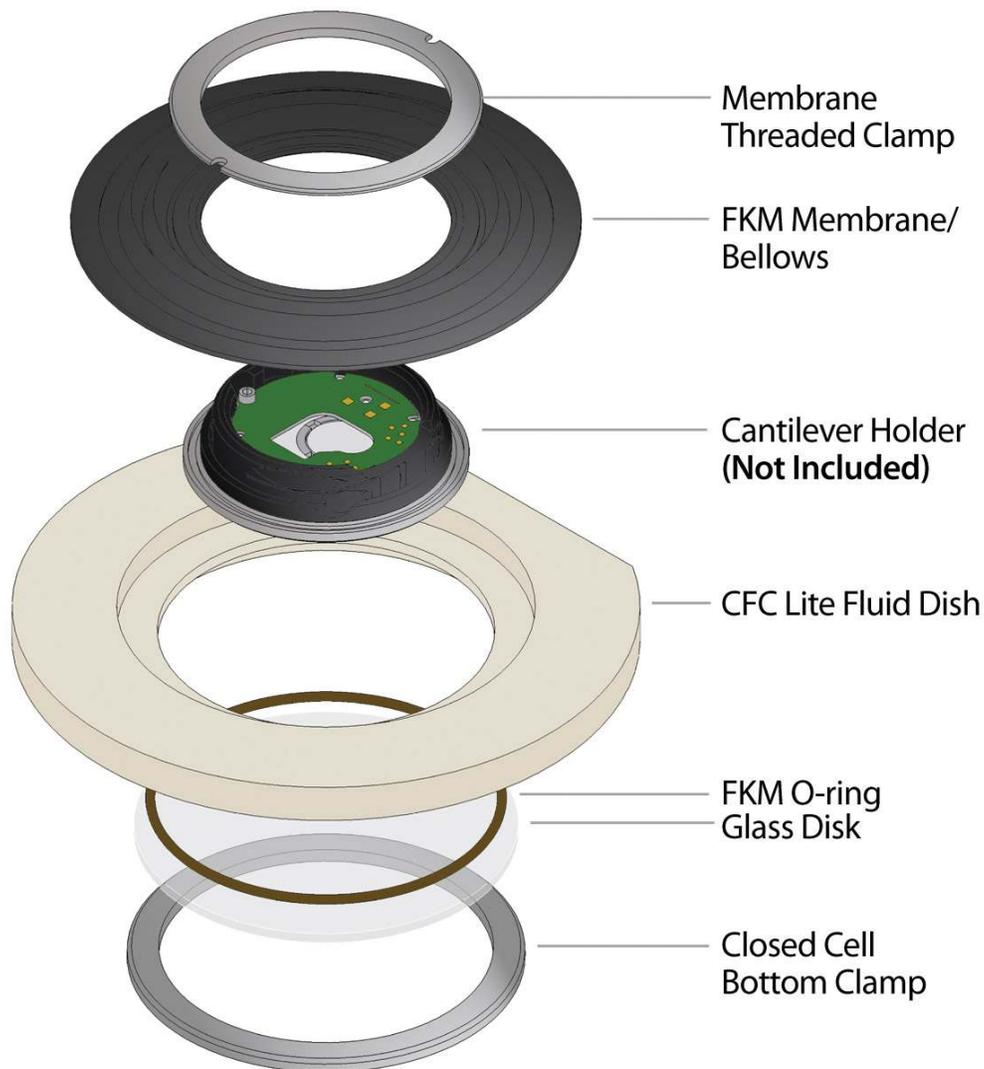
**Figure 13.2.:** Fluid Cell Lite components. SHOULD INCLUDE PART NUMBERS!!!!
