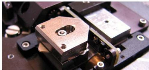
8. Repeat this process for the other pole face, making sure the two pieces are equidistant from the sensor bridge.
