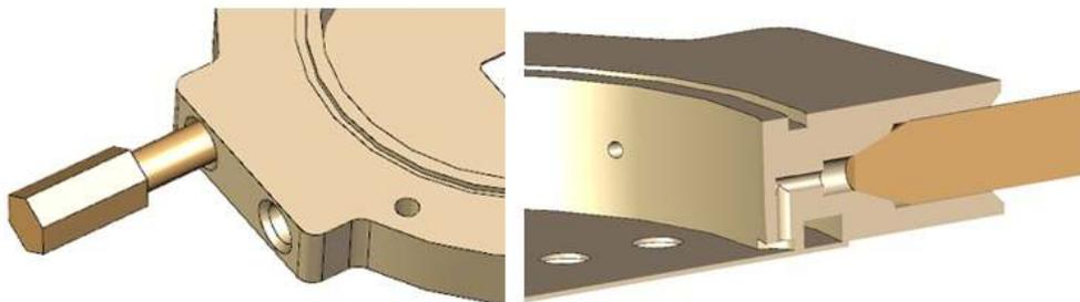
**Figure 24.9.:** A view of a fluid port fitting on the left. The cutaway view on the right shows the straight through port in the back (for fluid or wire feedthrough) and a cutaway of the fluid only port, designed to drain the fluid from the bottom of the cell.
