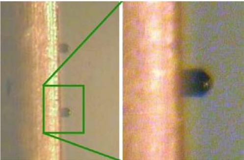
4. If the bubble is not removed after trying multiple times, lift the head up off the stage, place on its side and dispense some imaging liquid to remove the bubble with the force of the liquid under gravity.
