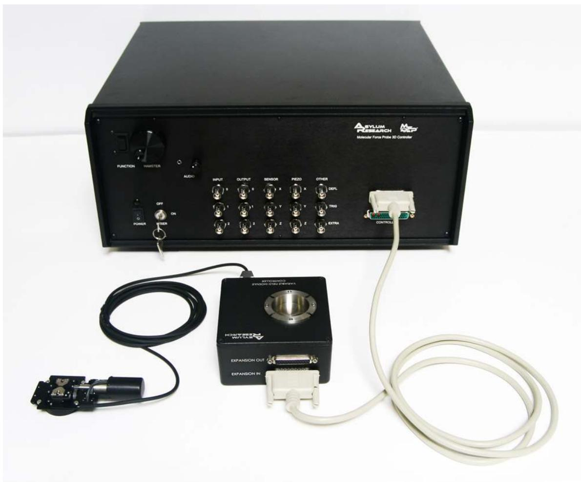
**Figure 25.2.:** The VFM sample stage plugs into the 9-pin connector on the VFM controller box. This in turn plugs into the 25-pin expansion connector on the front of the MFP-3D controller. This photo shows the older MFP-3D controller. The newer ARC2 controller can be used as well.
