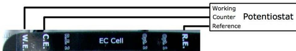
**Figure 24.12.:** Typical potentiostat connection scheme.
