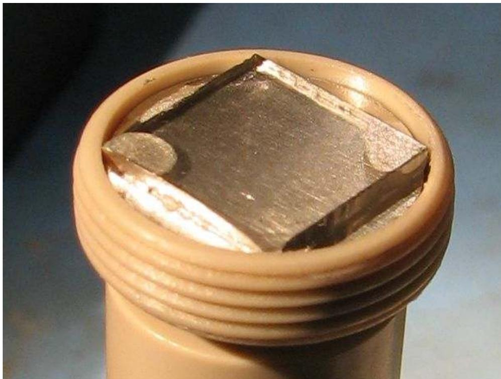
**Figure 24.6.:** Typical square sample of ITO on glass substrate. Note the dabs of silver paint at the corners which electrically connect the sample top surface to a metal disc carrier.
