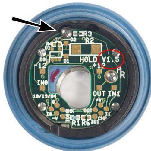
9. Clean the top of the glass insert from the upper side of the cantilever holder to remove any fingerprints from the reassembly. Use lens paper and alcohol.
