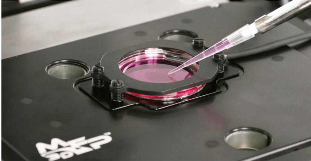
**Figure 23.5.:** Picture of Petri dish with clamp sitting on the scanner. Open access to the sample when the head has been removed.
