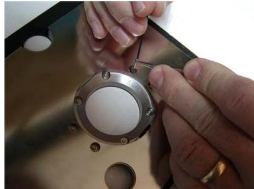
**Note** Scanners delivered prior to 2008 may be missing access holes for the outer screws. If this is the case, please contact the Asylum Research support department about obtaining a new cover plate with the access holes.
