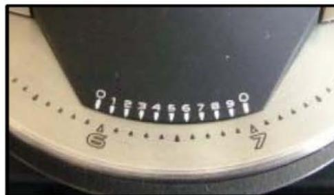
3. Once feedback has been activated, continue to lower the head with the front thumbwheel to  $\sim 70$  V (i.e. no color in Z-Piezo meter). This indicates that the piezo is in the middle of its Z- range ( $\sim 7.5$   $\mu\text{m}$  standard head;  $\sim 20$   $\mu\text{m}$  extended head).
