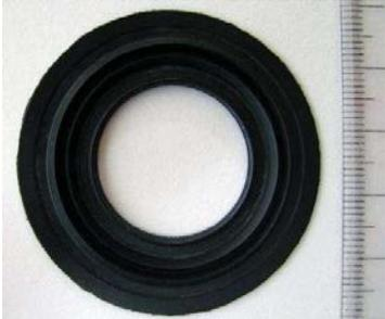
A black, circular, closed-cell bellows component, shown next to a ruler for scale.     |
