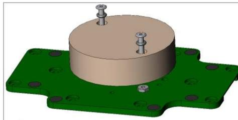
**Note** Do not overdo it on the tension. The Ring threaded bosses on the circuit board could tear off if overtightened.
