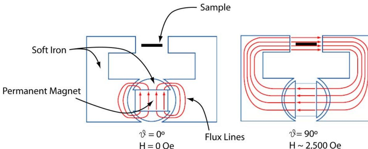
**Figure 25.1.:** How it works: A rare earth permanent magnet is at the heart of the VFM. The strength and sign of the magnetic field applied to the sample depends on the rotation angle of the magnet. When the magnet is at  $0^\circ$  or  $180^\circ$ , the magnetic flux is shunted away from the sample by the soft iron armature and pole pieces. As the magnet rotates, more and more flux is channeled instead through the sample. At  $90^\circ$  and  $270^\circ$ , the field magnitude is maximized.
