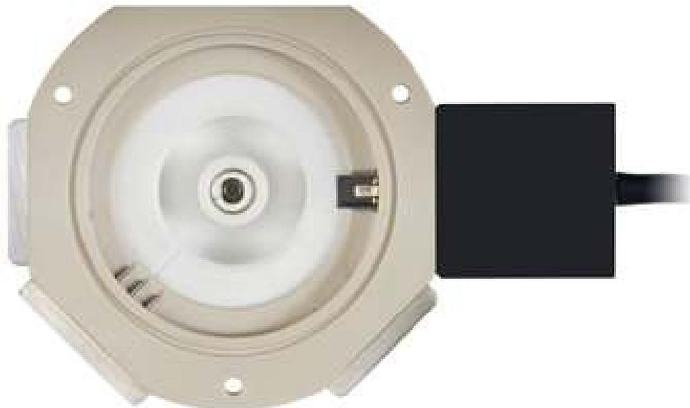
Figure 19.1.: Top View of assembled Humidity Sensing Cell.
