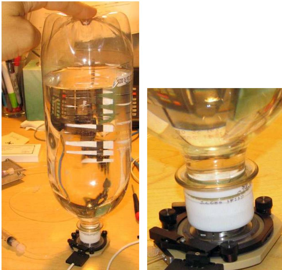
**Figure 14.6.:** Maximum pressure test by placing a weight onto a fully sealed closed fluid cell. Note the picture shows the Bioheater variation of the Closed Fluid Cell. Observe that the jaws on the clamp are OPEN to perform this test. Otherwise the clamp would support the weight of the bottle, and not the fluid inside.
