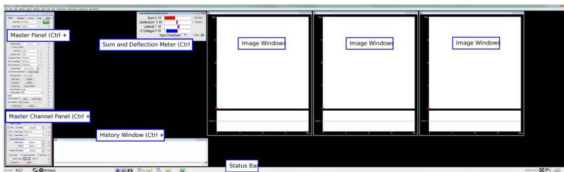
**Figure 3.1.:** Typical start up screen for the Asylum Research SPM Software, after the mode master panel has been closed. A few image panels have been left off the right of the screen, which usually extends across the second monitor of your system.
