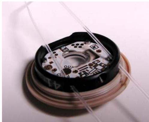
7. **Thread tubing into cantilever holder body:**
