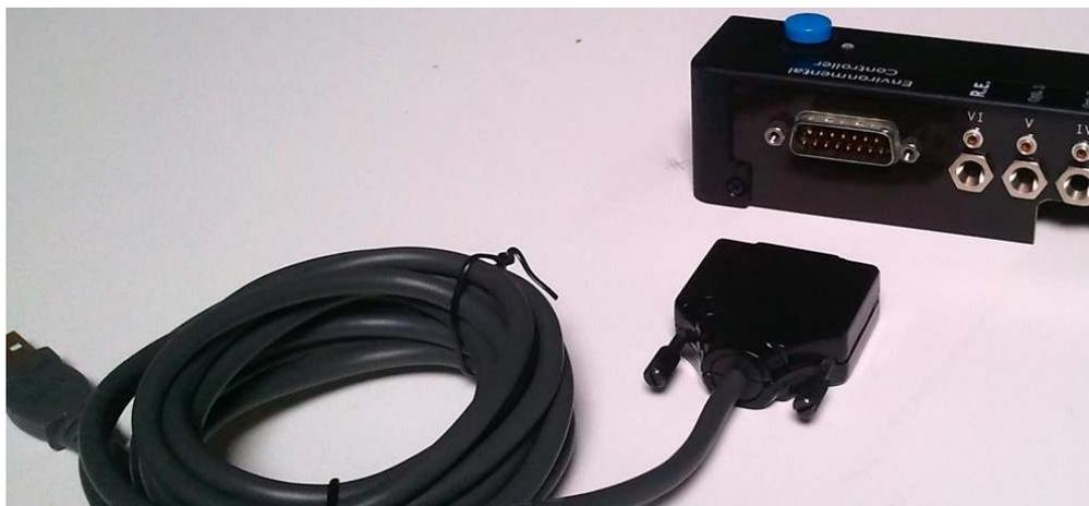
**Figure 24.18.:** Cable 448.130 supplies 5V to the junction box leak detection circuit. Plug one end into a free USB port on your PC, the other end into the junction box as shown.
