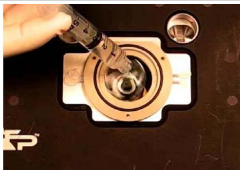
2. Prepare your cantilever for fluid imaging. Wet the cantilever with a bit of fluid as described in [Step 2 on page 69](#).
