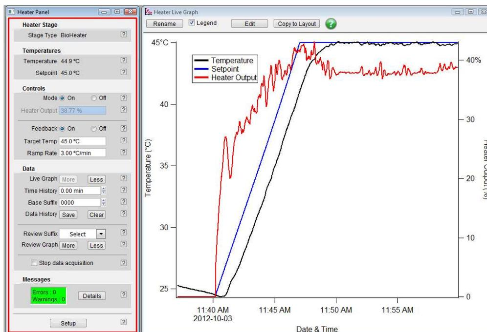
**Figure 17.3.:** Test of the Bioheater. What you might expect to see. Note that the temperature control will be less noisy if the cell is covered. You’ll discover this when using it inside the AFM.
