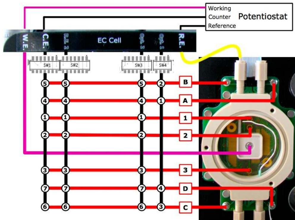
**Figure 24.16.:** Graphic which shows exactly how each dip switch connects the Junction Box connectors to the terminals on the EC Cell.
