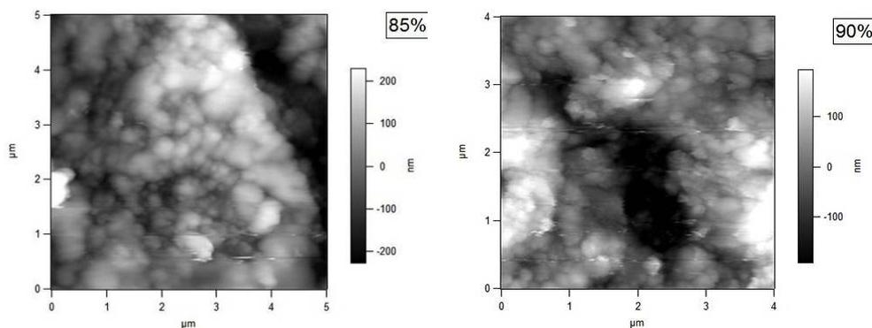
**Figure 18.6.:** Sample images taken in AC mode at temperatures approaching 400C.
