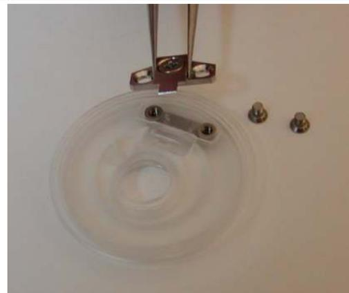
4. Clean the underside of the glass insert from the bottom side of the cantilever holder using camera lens paper and alcohol. Cotton swabs and tissues such as Kimwipes are too coarse and can scratch the glass surface and its anti reflective coating.
