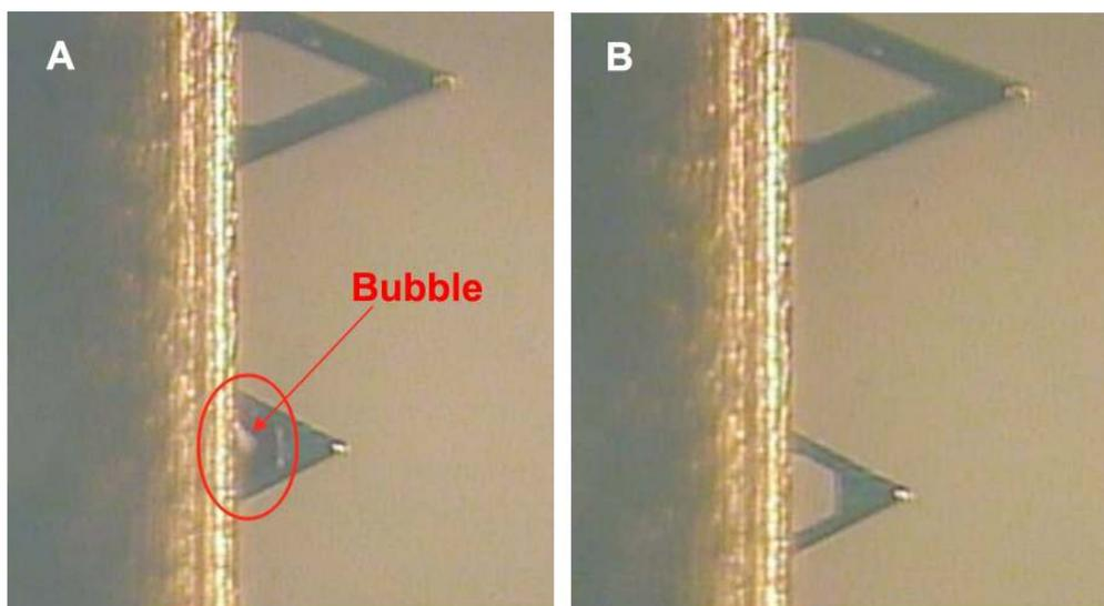
**Figure 8.4.:** (A) bubble trapped between the legs of a triangular cantilever, and (B) view with the bubble absent.
