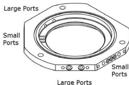
**Figure 14.5.:** 4 Large Fluid ports accept 1/16" OD tubing and 6 small ports accept 20 gauge hypodermic tubing or needles (0.036" OD).
