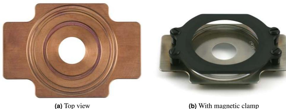
**Figure 22.1.:** Top (left) and side (right) views of the Petri Dish Holder. The photo on the right also shows the magnetic clamp holding down a glass bottom Petri dish.
