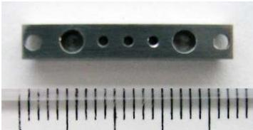
A rectangular, stainless steel closed fluid cell triple clamp is shown next to a ruler for scale. It has three circular ports on one side.                                            |
