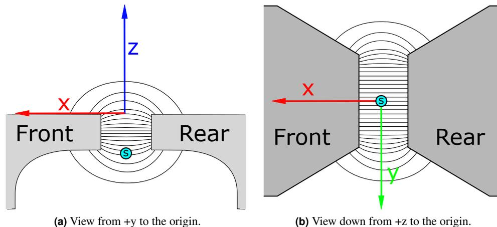
**Figure 25.5.:** Cartoons of the approximate fields between the pole faces. On the left, a side-view section, on the right a top down view. "s" denotes the position of the field sensor's active element. The origin was chosen at the optimal point for imaging. The central position of this point will maximize the field along x and minimize the other components. The origin also best mirrors the sensor position so the field measurement is as accurate as possible.
