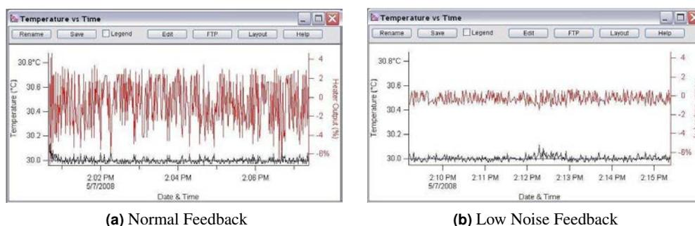
**Figure 20.7.:** Controlling Temperature near room temperature with and without the low noise option.
