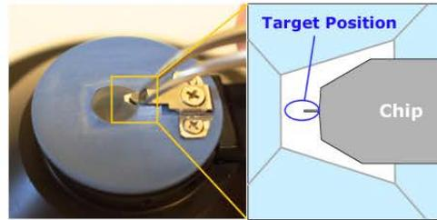
**Note** The quartz window is resilient to scratching from tweezers, so do not be paranoid.
