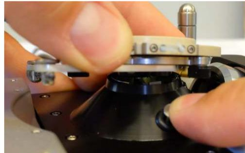
**Attach the assembly to the AFM head:**
