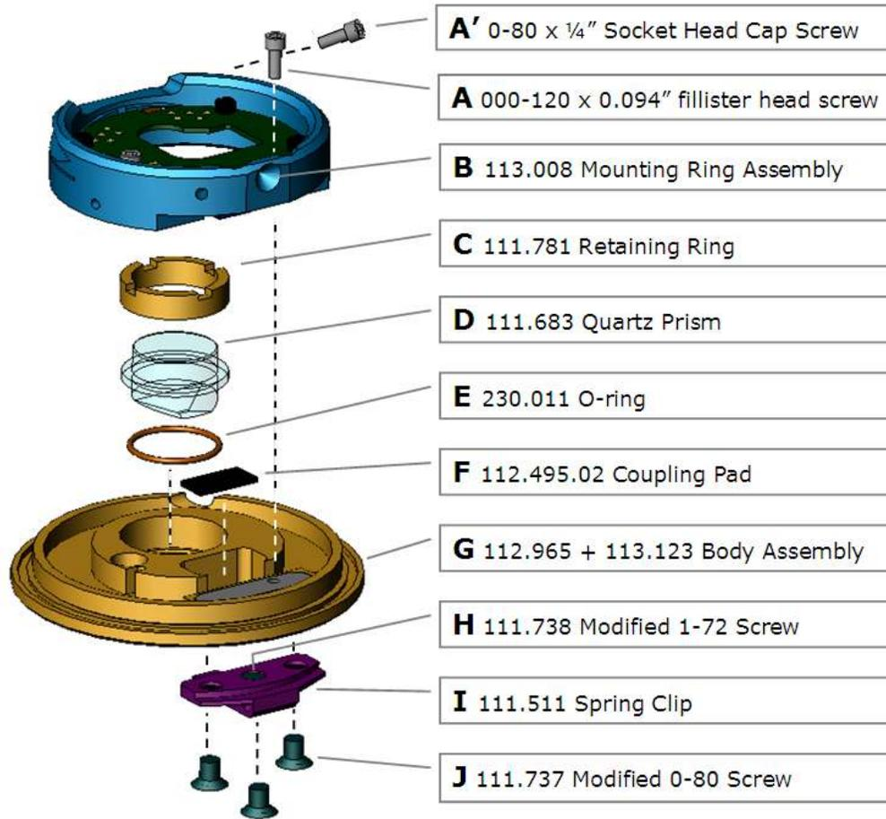
Figure 11.2.: Standard cantilever holder, exploded.
