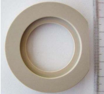
A white, circular, portless fluid dish is shown next to a ruler for scale. The diameter is approximately 4.5 cm.                                                                        |
